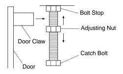
Figure 13 - Catch Bolt and Door Claw Orientation
